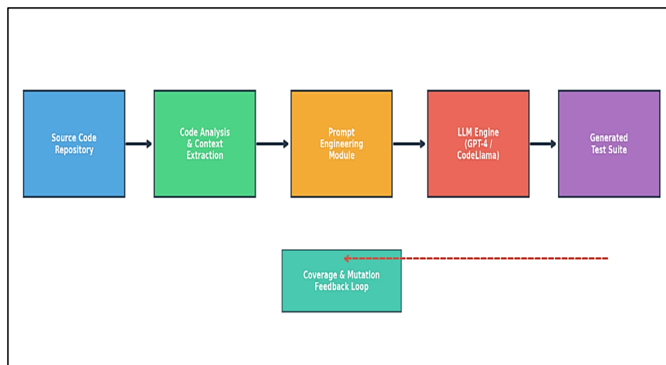
Fig. 1: LLM-Test pipeline: source code analysis, prompt engineering, LLM-based generation, and coverage-guided feedback loop.
